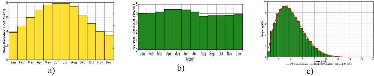
Fig. 5 Average global solar radiation (kw/m<sup>2</sup>/day), b) Wind speed (m/s), c) Wind speed probability distribution of Ghardaia.
